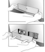
To change setups using shorting bars, use the supplied hexagonal driver to remove the screws
